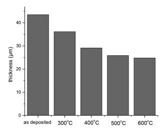
FIGURE 3. Thickness of TiO, thin film annealed at different temperature
