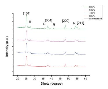
FIGURE 2. XRD spectrum of TiO<sub>2</sub> thin films annealed at different temperatures
